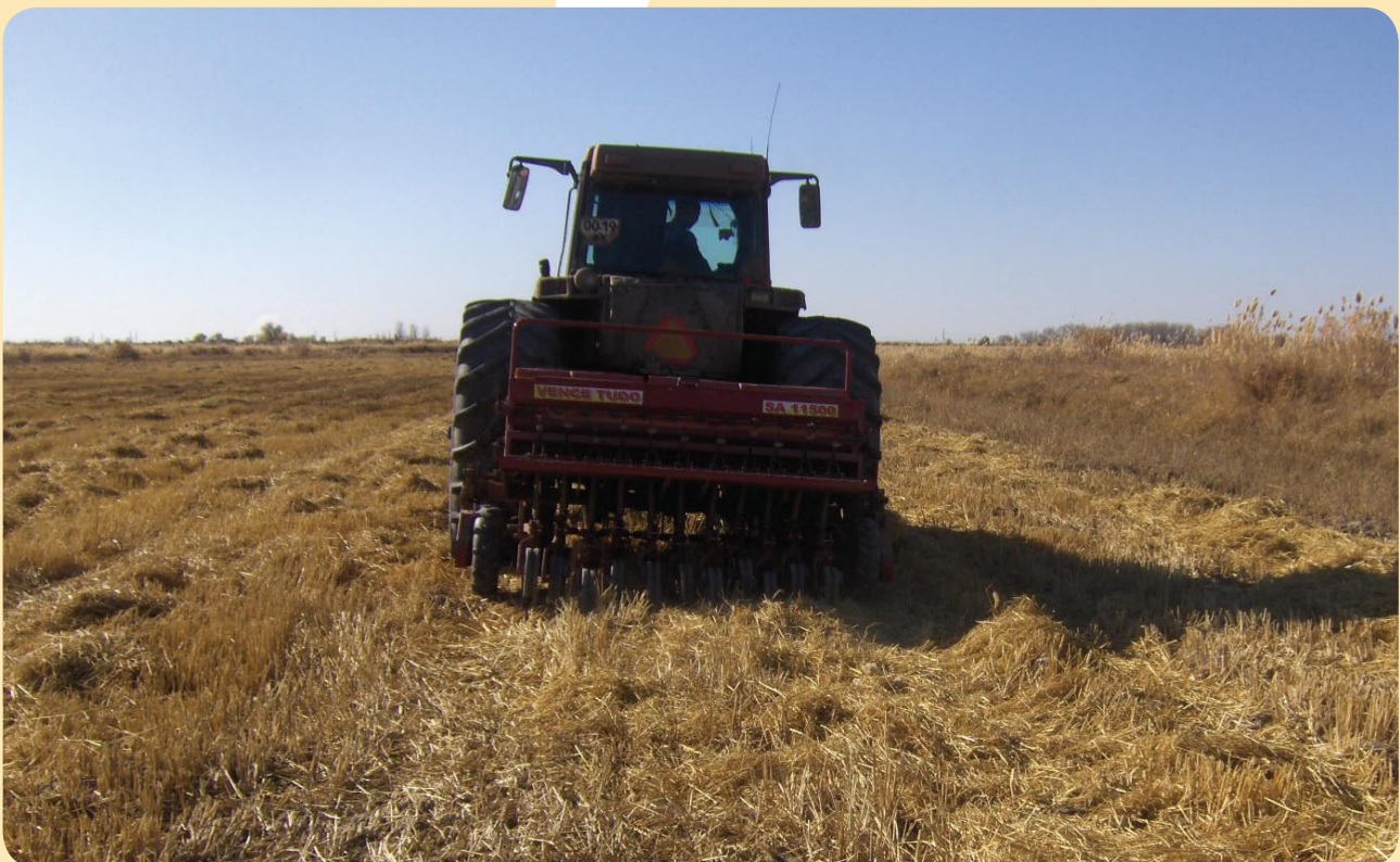
Photo 2. No-tillage experience in Karakalpakstan. A direct mulch seeding
